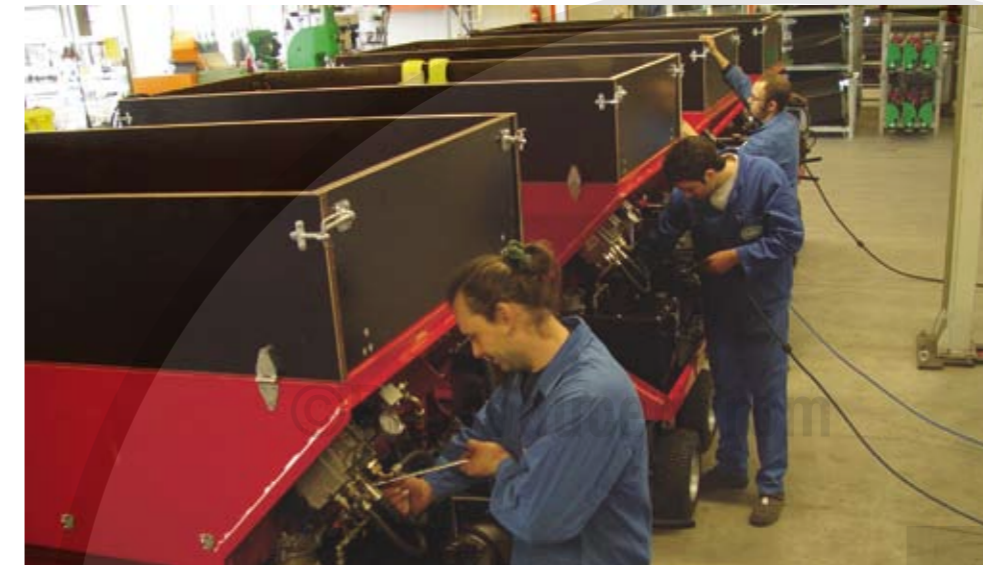
SandMatic machines – used for scattering artificial turf infilling material – in the assembly hall
