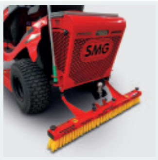
Brushes with plastic bodies, can be changed without tools
