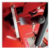
**PRECISE:** Manual outlet lever for precisely adjusting the infill quantity.
