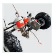
**FLEXIBLE:** Pivoting cutting unit for the trimming of artificial turf or cutting marginal areas.
