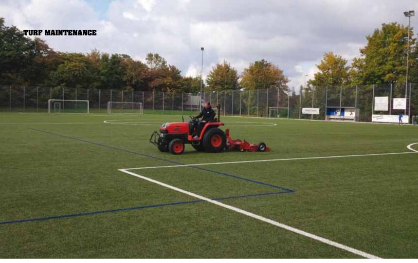
(Above) SMG's TurfCare TCA1400 is a ground driven, tow-behind device for artificial turf cleaning and care (Below) The SandMatic B1505RC is a self- propelled, radio-controlled machine for the filling of artificial turf
